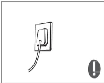
The power plug should be firmly plugged into the socket. Please ensure that the grounding electrode of the power socket is accurately grounded.
