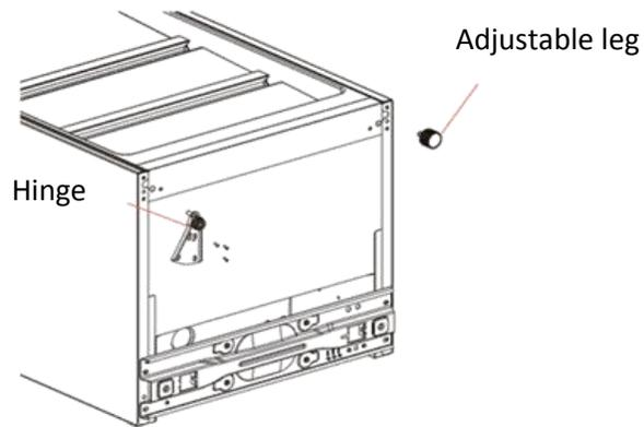
7) Mount the door on lower hinge, vertically, and make sure the door gasket is tight, take out the spare upper left hinge and hinge cover (included in the accessory bag), then install the upper left hinge using the fitting screws. Finally install the hinge cover, and the hinge hole cap on upper right side.
